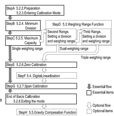
Step H Gravity compensation function. Perform this function after span calibration.
