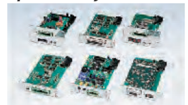
Top Row: DeviceNet, RS-232C and CC-Link Bottom Row: RS-422/485, Analog output, and PROFIBUS
