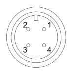
Pin GND, Signal Ground
