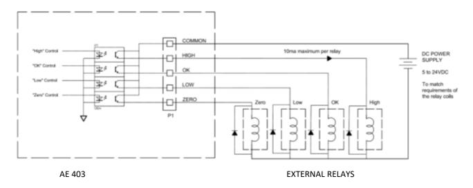
Connections are made to the PCB, Connector P1. The connector is a spring activated type, simply press on the top of the connector and insert the wire.
