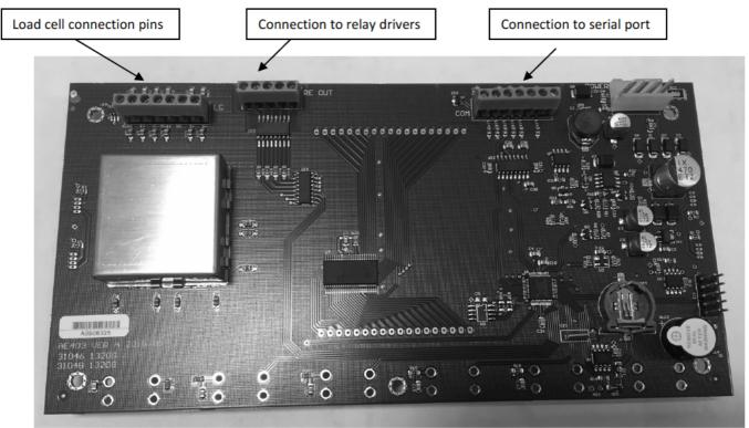
FIGURE 5 AE403 CIRCUIT BOARD
