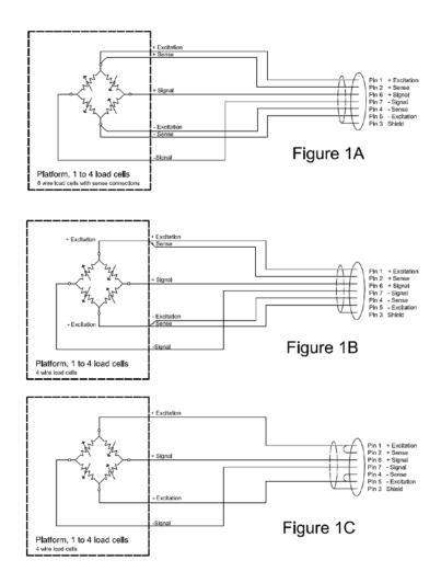
Figure 1A shows the connections to a 6 wire load cell. Figure 1B and 1C show 2 different ways to attach a 4 wire load cell, 1B uses a 6 conductor cable to go from the indicator to the platform or load cell where it connects to the 4 wires from the load cells.
