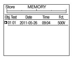
If the screen does not display the measurement and **pressing the MEM key has no effect**, press the **DISPLAY** key twice to restore the result screen, then press the **MEM** key again.
