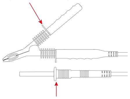
Measurements of voltages ≥1000 V on supply lines should be made using the test probes only, with the user's hands behind the hand guard on the lead.
