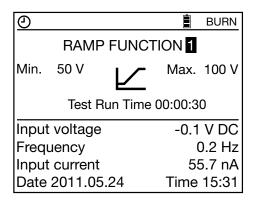
Use the ▲ ▼ buttons to select a preset test voltage ramp:
