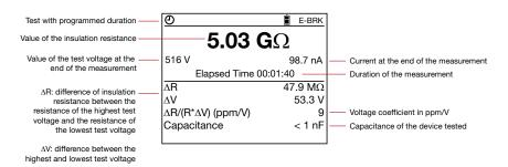
Record the measurement and compare it to earlier measurements in order to assess the evolution of its value. Also record the temperature and the ambient relative humidity.
