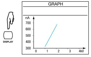
This curve is useful primarily in the case of a measurement in V-RAMP mode. There is no cursor and it is not possible to zoom on this curve.
