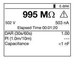
The **DISPLAY** button is used to look up all information available after the measurement. This information depends on the type of measurement chosen (see § 2.4.4).
