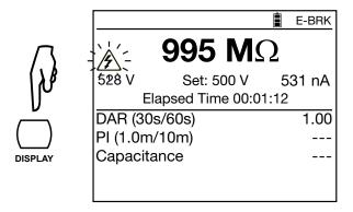
In the case of a step test voltage (10 steps at most) or ramp test voltage (3 steps), the progress of the steps will be indicated.
