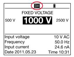
The High setting is recommended when measurements are made in the presence of strong electromagnetic fields at the network frequency (for example near high-voltage lines).
