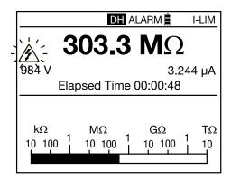
The **FILTER** button can be used to activate and deactivate a digital filter for the insulation measurements. This filter affects only the displayed results (which are smoothed), not the measured values. The recorded data therefore remains raw (no filter).
