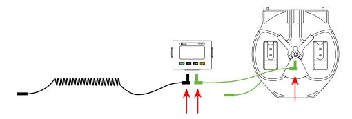
Add the crocodile clip and the probe tip on the ends of the leads.
