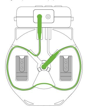
■ Hook the take-up reel onto the belt, then hook the strap to the take-up reel and adjust. Your hands are free to hold the probe tip.
