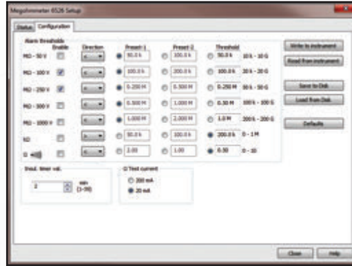
Configuration screen allows you to set alarm levels, test time and to read and write configurations from and to the instrument.
