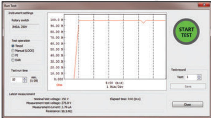
Select test conditions and start a test from the PC and display real-time measurement results graphically.
