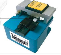
Compact design, lightweight and robust. Ideal for FTTx applications on-site. For 125  $\mu$ m diameter fibers. Blade life for 12,000 cuts. Fiber holder by springs with magnets.
