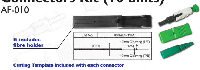
The SC / APC connectors Kit provided by **PROMAX** is delivered in a 10 unit batch. To make fibre optic connectors easy to install on field, it includes a holder and a cutting template printed to actual scale. The connectors kit includes 10 fibre holders and 10 cutting templates, one per connector.
