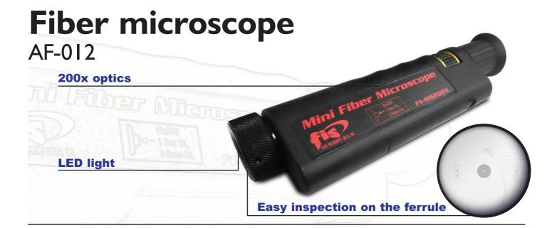
200x microscope designed for inspecting fiber ends, to look for dirt, impurities and oils that might interfere with signal transmission. It includes a universal 2.5 mm adapter for inspecting ST, SC or FC connectors, as well as a 1.25 mm adapter to inspect LC ferrule connectors. This microscope uses an oblique and coaxial LED light (powered by 2 AA batteries, included). Padded included.
