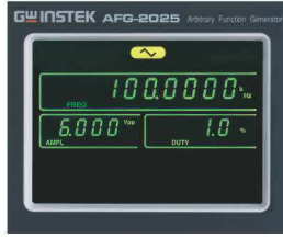
1% Duty Cycle of Square Wave Setting
