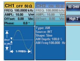
50Ω / High Z Impedance Switch Function
