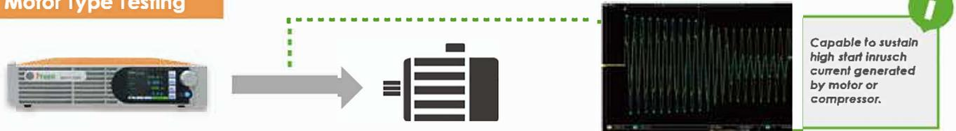
AFV-P series can deliver up to 4.5 times of peak current from its RMS current, and it can control the product output according to user-defined start/end angle, so it is suitable for testing switching power supplies with high inrush current issue. Additionally, it is able to provide a customized 150% overload capability for starting up motor-type DUT, such as electric motor.
