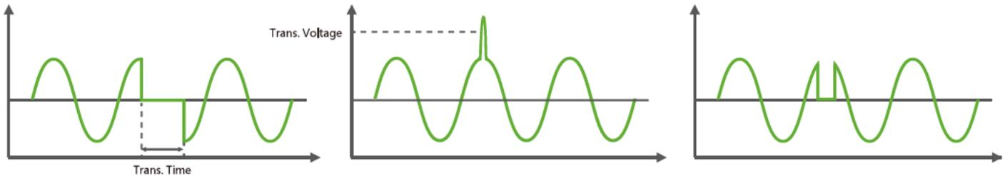
With the Transient feature, user can have more control over the output waveform by adding disturbance at user-defined locations with user-defined drop/rise range. This feature is useful to simulate different pre-compliance test and various types of power line disturbance, such as surge, sag, spike and dropout, for immunity tests.
