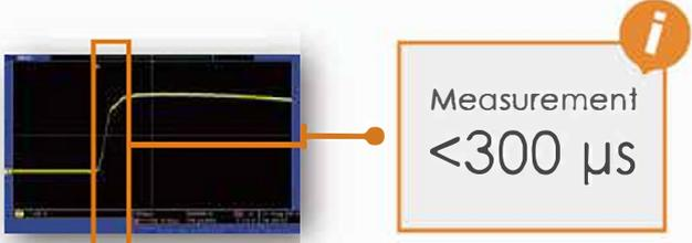
To simulate power line disturbance, such as sags, surges, dropouts and spikes, response time has always been a critical factor. AFV-P series is a high performance AC source with fast response time less than 300  $\mu s$ , and users are allowed to do pre-compliance tests accordingly, such as IEC-61000-4-11.
