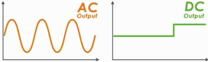
AFV-P series can selectively generate AC output or DC output according to user-defined settings. This feature not only extends applications to AC & DC component test, but allows effectively cost reduction of purchasing another DC source. Therefore, it is an ideal power testing solution for R&D unit and certification laboratories with limited space.
