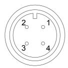
1: Pin GND, Signal Ground
