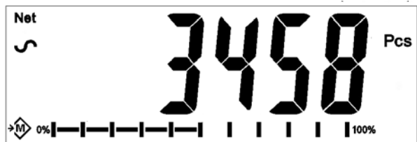
Checkweighing during Parts Counting
