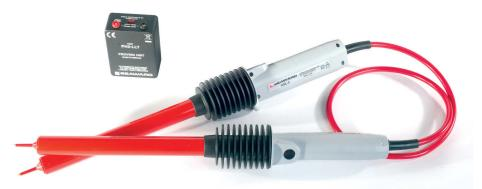
The Seaward AGL-5 is a two pole voltage detector designed specifically for use with airfield ground lighting systems. The instrument indicates the presence of voltages greater than 50V AC and is ideal for proving dead on AGL systems up to 5000V. The unit is totally encapsulated in a high impact rugged enclosure and is IP64 rated. The ultra-bright high intensity red LED indicators and a polarizing filter make it clearly visible in all working environments.
