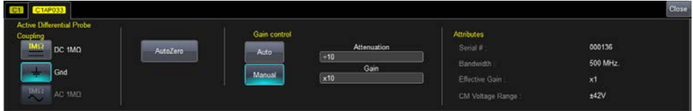
Figure 5, AP033 probe dialog with probe controls and attributes.
