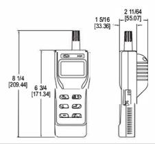
The **MODEL AQH-20** Handheld Indoor Air Quality Meter reduces he number of instruments a contractor has to carry by measuring carbon dioxide concentration, air temperature, and humidity percentage in one device. A large backlit LCD shows all three parameters simultaneously. This product offers user selectable engineering units, maximum/minimum/average readings, a hold func ion, and an audible alarm.
