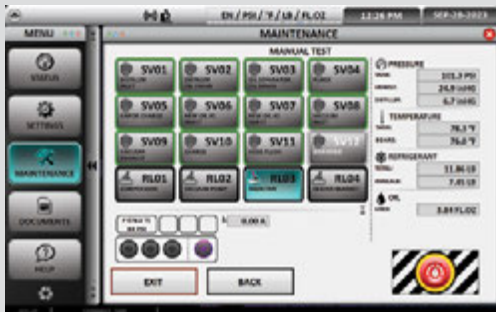
Maintenance Screen offered only to authorized service technicians allowing for quick and easy diagnosis
