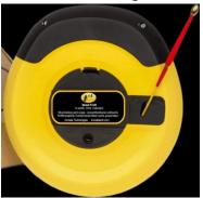
track the path up to 98 feet of non-metallic pipe or conduit buried in the ground or routed in walls. When used in conjunction with wire trackers like the Armada 33 kHz Pro290™,Pro881™, or Pro900™ it is possible to determine the route of PVC or vinyl conduit. The Pro66 does not require batteries.
