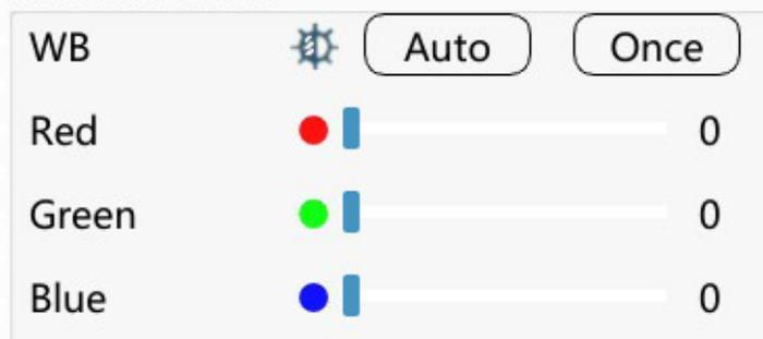
Place a white card under the microscope, adjust the focus, and click on "Auto"
