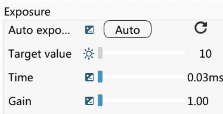
When Auto Exposure is enabled, the target exposure can be set by sliding the "Target Value" bar to the desired value.
