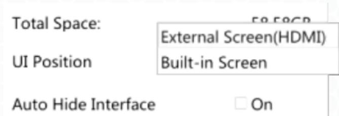
*\*The live on-screen image will show up on both monitors while in HDMI mode, however the user interface (UI) will only show up on either the **Built-in Screen** or **External Screen (HDMI)**. Choose which screen you want the UI to display on by clicking the **UI Position** drop-down menu under the settings tab.*
