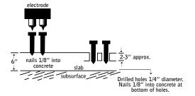
If the meter still indicates green or "dry" the floor is ready for covering. Tests should be made at several points, especially when the slab is thick and air circulation is poor. Tests should only be made in newly drilled holes, since the inside surface of the holes can dry out while the rest of the slab is still wet.
