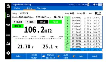
Discharge testing: measure cell impedance, voltage, and temperature
