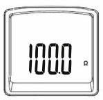
If the loop impedance is  $1000\Omega$ , then the  $2000\Omega$  range must be selected, and the test result display like the below screen.
