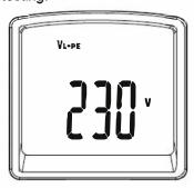
If the voltage is less than 150V then the "Lo" Symbol will be displayed on the screen.
