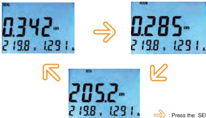
→ : Press the SELECT button can see REAL/HOUR/MTH kWh.
