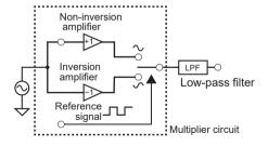
Where the reference signal voltage of the AC current generated in the instrument is v1, the signal voltage for use in synchronous detection is v2. These parameters may be expressed by the equation given below. A phase difference from vi, due to a reactance component, is represented as  $\theta$  in the equation for v2.
