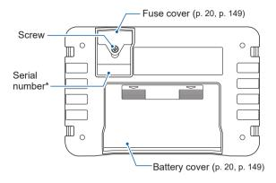
\*: The serial number consists of nine digits. The first two (from the left) indicate the year of manufacture, and the next two indicate the month of manufacture. Required for production control. Do not peel off the label.
