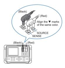
When using the 9460 Clip Type Lead with Temperature Sensor (option), connect the mini plug to the TEMP.SENSOR terminal. See "3.9 Measuring Temperature" (p. 68).
