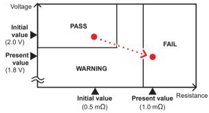
As shown above, this battery needs replacing.
