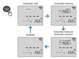
To disable the hold function, press the **HOLD** key or the **PRESS** button on the 9466 Remote Control Switch.
