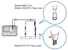
Insert the pins with the marked (engraved) side of the probe facing you.
