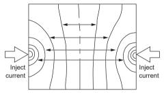
Figure 1: Equipotential lines on a metal plate, showing the current distribution at 50 µV intervals when a current of 1 A is injected from the distal points of the plate (W300 × L370 × t0.4)
