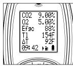
02/Eff displays 02 (%), Gross Efficiency, Flue Temperature.
