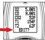
AUX displays 5 lines of editable parameters. To edit line values Press ▼ button until **Edit?** displays on the Status Bar. Press and Hold ← until the
