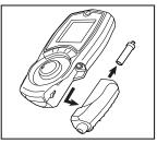
Remove protective rubber boot. Remove water trap from analyzer. Remove particle filter from spigot and replace with new one. Reattach trap and boot.
