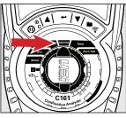
Rotate the function rotary dial to CO/CO2 for Test Screen 2 parameters.
