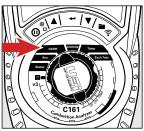
Rotate function rotary dial to 02/Eff for Test Screen 1 parameters.
