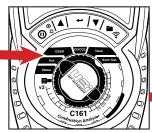
When performing a combustion Test, Rotate function rotary dial to AUX to view the Auxiliary Test Screen's custom parameters.
