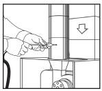
Remove the probe from the flue and allow analyzer to purge with fresh air until readings return to zero. 02 to 20.9%, CO to Zero **CAUTION:** probe tip will be HOT.
