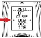
Rotate the dial to MENU. Press button until the LOGS is selected between two arrow icons. Press to select.
