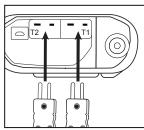
Insert K-type temperature probes into input T1 and T2.
