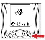
To Log: During testing, Press and Hold row to log a report. To view these Logs, see **View Saved Logs** section.
