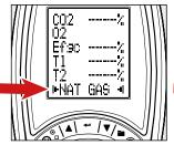
Press ▼ button until the Fuel Type displays on the Status Bar. Press and Hold ← until two arrow icons display.
