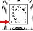
To print the LOG, Press ▲ and ▼ buttons until PRINT is selected between two arrow icons. Press ← to select to start printing.
