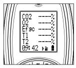
O2/Eff displays CO2, O2, Gross Efficiency, Flue temperature, Inlet temperature.
