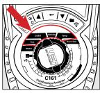
Rotate the dial to either AUX, 02/Eff, C0/C02 or TEMP setting.
