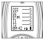
02/Eff displays C02, 02, Gross Efficiency, Flue temperature, Inlet temperature.
