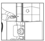
Insert flue probe into stack. Adjust cone so the probe tip is approximately at the center of the stack.
