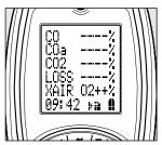
CO/CO2 displays CO (ppm), Losses calculated, Excess air %. Make any adjustments needed for proper Combustion and wait for analyzer to display change in readings. (Repeat as necessary).
