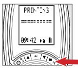
During testing, Press 훆 to start printing.
