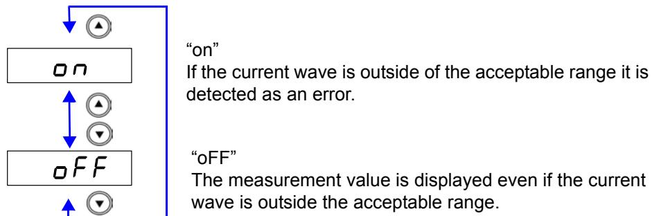
4. Press **[ENTER]** to confirm the current detection circuit monitoring function as enabled or disabled.
