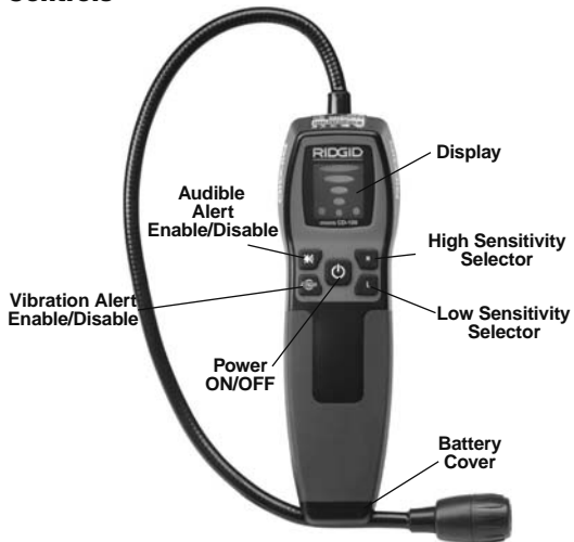
Figure 2 – micro CD-100 Parts
