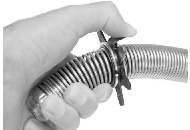
Figure 19 – Pre-stress tabs by placing your finger at the top of the spike and slowly pushing the spike 90 degrees. Repeat in the other direction.
