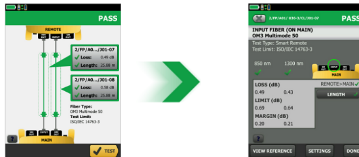
Complete data is displayed with a test result. The dotted line shows what's included in the measurement. Detail windows show the results for each fiber tested.
