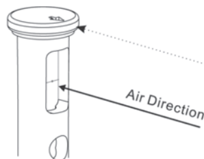
Fig. 6. How to orient the hot wire probe
