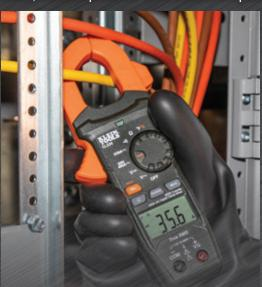
HVAC 400A AC TRMS CLAMP METER WITH TEMPERATURE AND DC MICRO AMP
