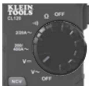
2. Apply test leads to the circuit to be tested to measure voltage. The meter will auto-range to display the measurement in the most appropriate range.
