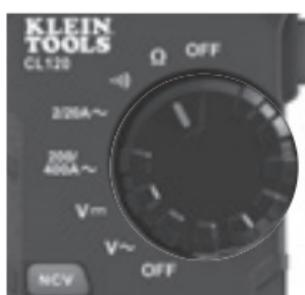
**NOTE:** When in a Resistance setting and the test leads are open (not connected across a resistor), or when a failed resistor is under test, the display will indicate O.L. This is normal.
