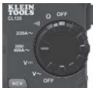
2. Place clamp around wire. The current measurement will be shown in the display.
