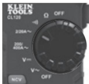
**⚠** *Disconnect test leads when measuring with the clamp.*
