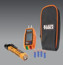
RT250 is an electrical receptacle tester with LCD that identifies common wiring faults on North American 120V outlets. The LCD displays the voltage, identifies the wiring fault, and the time required to trip a GFCI device.
