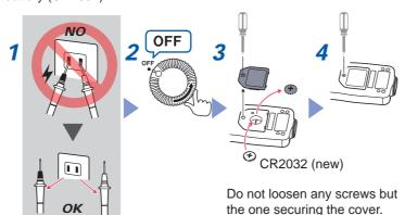
Do not turn any one of the 3 screws inside the battery case. Doing so will cause the instrument to report abnormal measured values.
