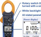
Rotary switch that can be turned with a single hand
