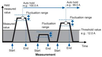
If the measured value falls below the threshold value (voltage, current) or exceeds the threshold value (resistance, continuity, diode) after display value updates are stopped, display value updates will stop once more if the two conditions are satisfied again.
