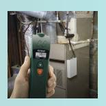
Check CO levels up to 999ppm with the push of a button using Model CO15. An audible alarm indicator will continuously beep starting at 25ppm (preset warning level - value can be adjusted) and the display will flash until the CO level goes down to normal range. A backlight on the display can be used for low light areas. The meter comes complete with batteries, wrist strap, and pouch.
