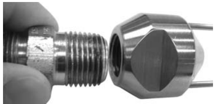
Figure 4 – Installing Adapter Into Cone
