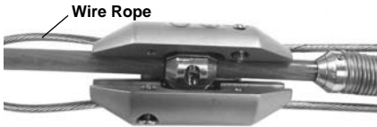
Figure 6 – Locate Pushrod Bulb In Shell
