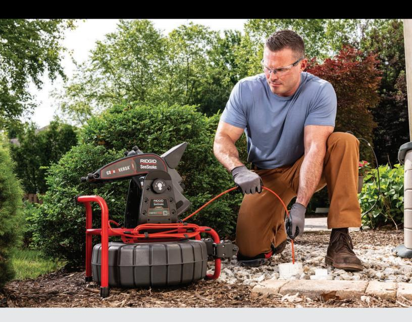
The RIDGID® SeeSnake® CS6x Versa™ is the flexible, efficient solution for plumbing inspections. The CS6x Versa works with all SeeSnake camera reels and easily docks onto Compact series reels. The frame allows the monitor to be tilted to the optimal viewing angle, and a quick-release mount lets the monitor be placed in a high or low viewing position to suit jobsite conditions.
