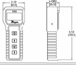
The **MODEL CSG** Current/Voltage Signal Generator generates a 0 to 10 VDC signal in increments of 1 V or a 0 to 20 mA signal in increments of 1 mA. The large LCD features a blue backlight for use in dimly lit areas. Model CSG continuously ramps the output using the user selected minimum, maximum, and ramp interval timing parameters.
