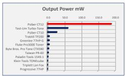
Output Power measured into a 600 Ohm load.
