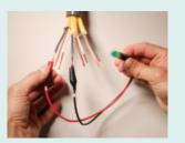
GREEN LED means wiring is properly identified.
