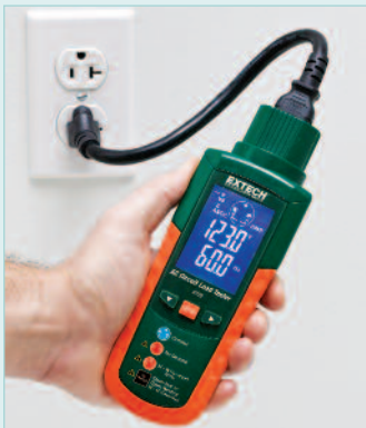
Tests 3-wire standard and GFCI receptacles
