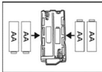
5. Push the loaded magazine back into the grip (it fits only one way).
